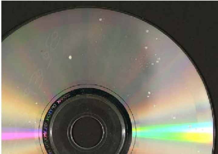
Image 1. Disc showing disruption of the metal reflective layer after accelerated aging
