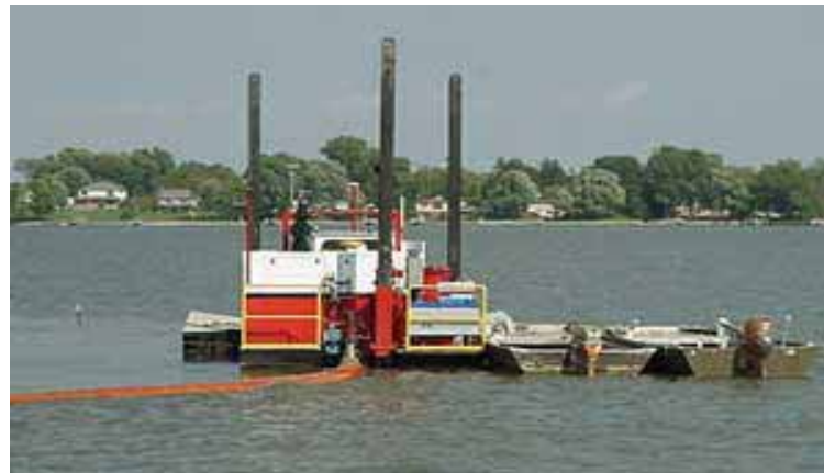
Dredging equipment used to clean up contaminated sediment in Little Lake Butte des Morts.
