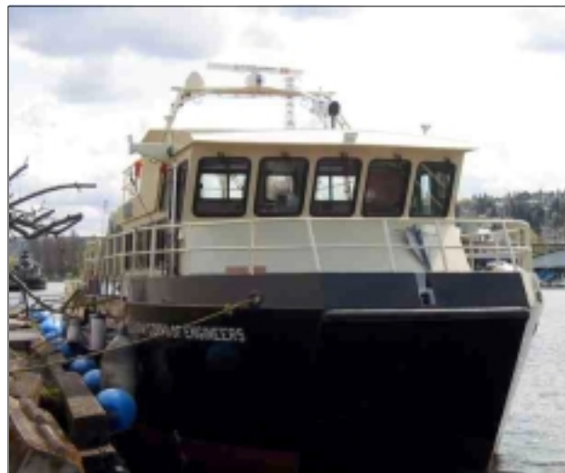
The Moritz pierside in Washington. The vessel is 58 feet in length, with a beam of 18 feet, six inches, displaces approximately 30 tons, and can sustain speeds of up to 30 knots.
