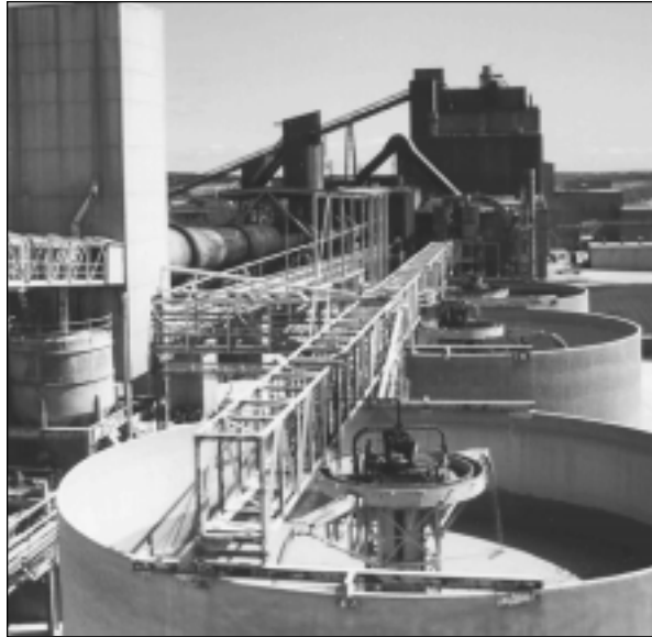
▲ The Passamaquoddy Technology Recovery Scrubber™ was successfully demonstrated at Dragon Products Company's cement plant in Thomaston, ME.
