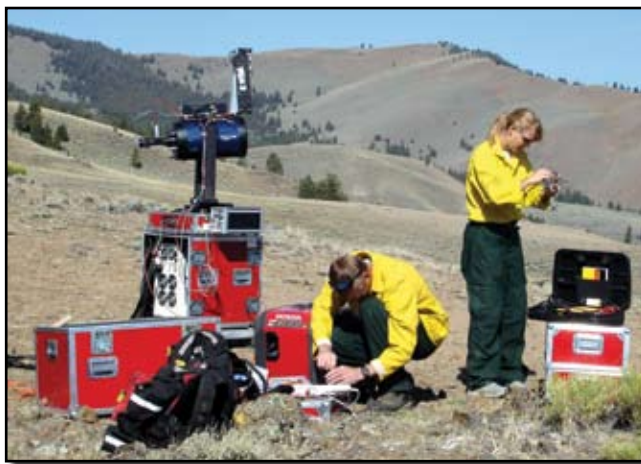
The mobile lidar equipment measures the optical properties of aerosol particles in real-time over a large area.
