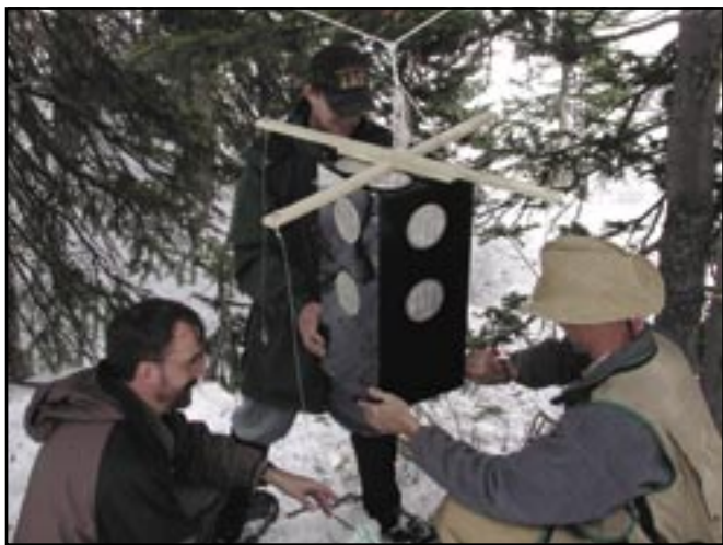
To help assess the extent of spruce beetle populations, researchers built and installed traps baited with infested green tree bolts.
