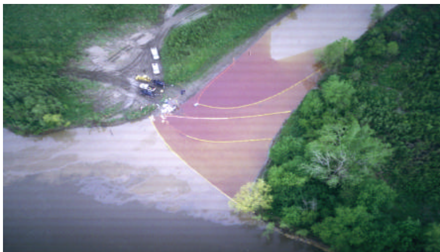
Containment booms were set up on the mouth of Independence Creek to prevent further contamination of the Missouri River.
