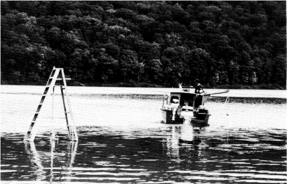
Figure 14. Current meter setup in the field
