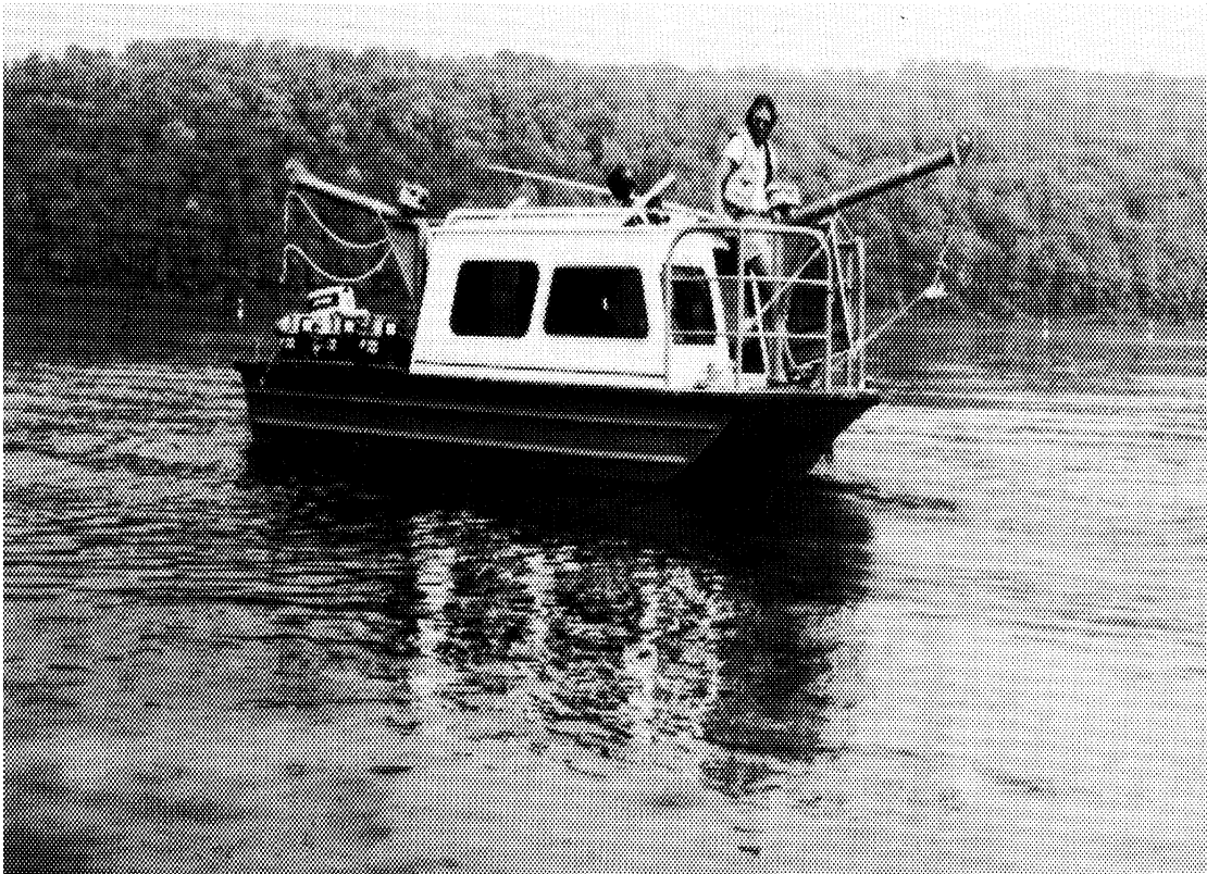
Figure 4. The Water Survey research boat "Monitor" with sampling booms at the bow and stern
