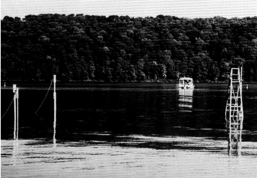
Figure 15. Setup of wave gages and current meter in the field
