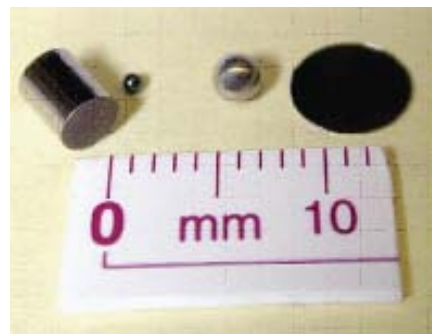
Figure 1: Pt cylinder, YIG sphere, Ni sphere, and Ni disc SRMs.
