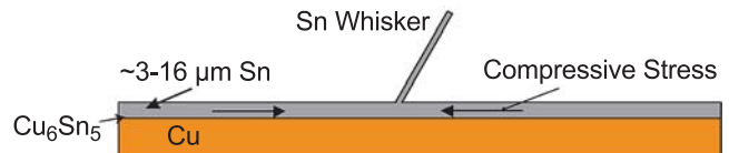
Figure 2: Schematic of Sn whisker growth from a Sn electrodeposited plating.
