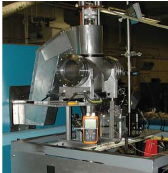
Figure 1: Small scale Laval atomizer for production of 250 g lots of metal powder.
