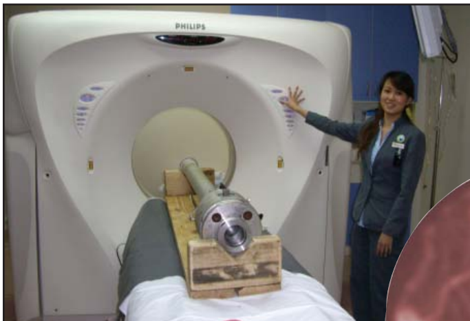
Pressure core being X-ray CT scanned at the Gleneagles Hospital in Singapore.
