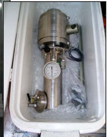
A 20-cm subsection under pressure in a transportable Parr vessel.
