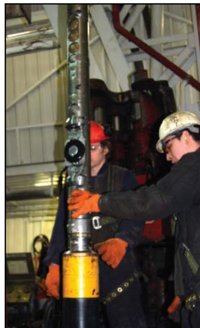
The Doyon 14 crew rigs up Schlumberger's Modular Dynamic Tester
