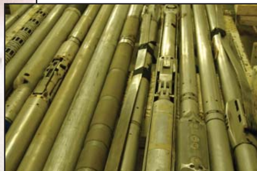
Logging tools: the science effort included a research-level open-hole wireline well logging program
