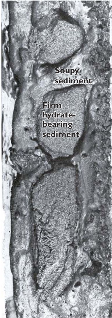
Figure 1. Dissociating sample of a marine HBS core. (Deep Sea Drilling Program, Leg 67, courtesy of C.K Paull of the Monterey Bay Research Institute).
