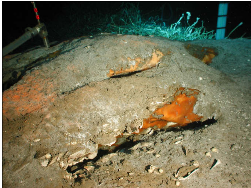
The gas hydrate mound has a thermistor probe installed. The location is GC185 at a depth of 1800 ft (545 m). The picture was taken with the time-lapse camera deployed by the GHOSTS program.
