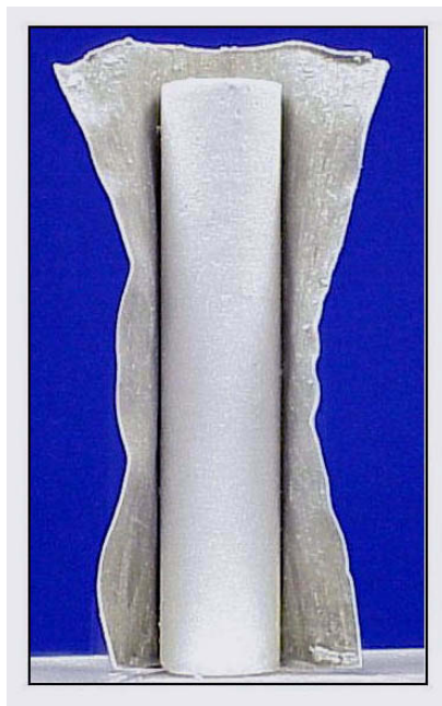
The left photo shows a full methane hydrate sample in a split metal jacket. The right photo shows mixed-sand/methane hydrate mixtures stratified with different proportions of sand and hydrates. The yellow layers are made with quartz sand and the gray layers with aluminum oxide. A translucent Teflon sheath surrounds the two samples to the right.
