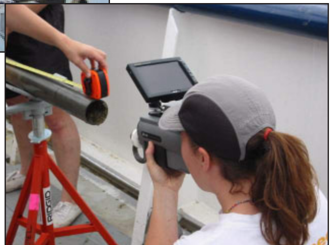
Graduate student Jill Weinberger (Scripps) acquires an infrared image of the end of a recovered piston core.
