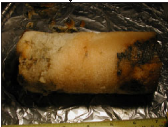
A 9- by 22-centimeter core of gas hydrates is collected with the hydrate drill.
