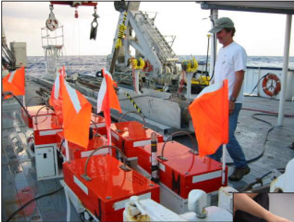
The osmotic flux meters on deck with Mike Tryon (Scripps) following retrieval at Bush Hill.
