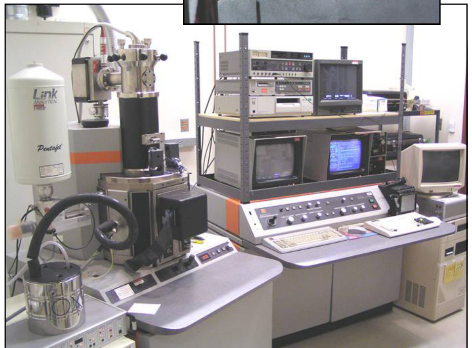
ElectroScan Model E3ESEM located in the Environmental and Molecular Sciences Laboratory at PNNL
