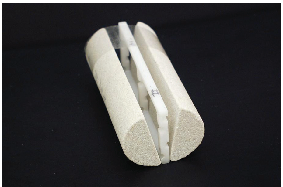
Figure 1: Halves of Bentheim sandstone core fitted with a 4 mm thick spacer of POM that was used for many of the hydrate formation and production tests.
