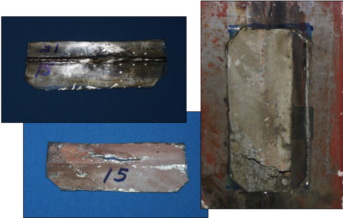
Figure 5.88 Liner Specimen at Tear #15
