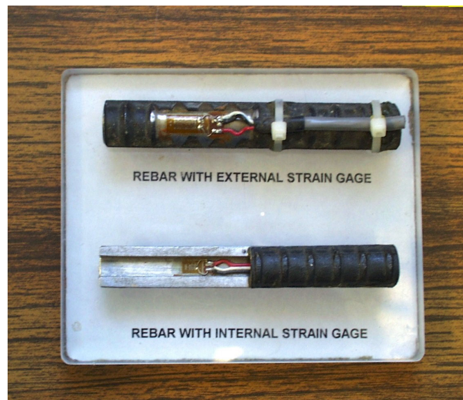
Figure 3.9 Sample Rebar and Gage Bar Strain Gages
