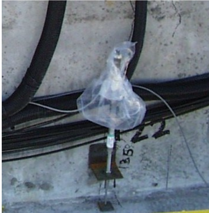
Figure 3.5 External LVDT Measuring Displacement between Basemat and Mudmat
