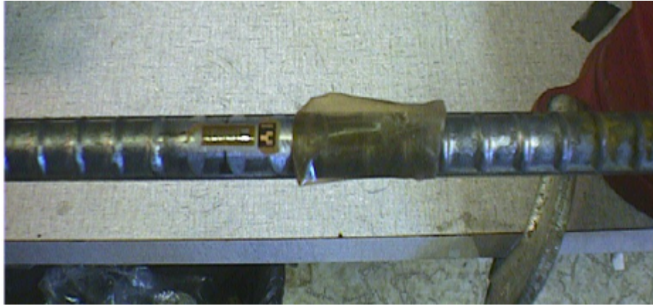
Figure 3.6 Rebar Strain Gage
