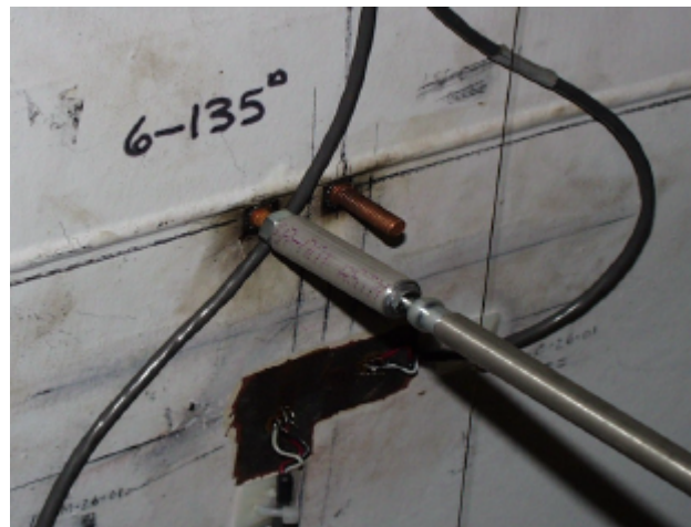
Figure 3.4 TLDT Mounted on Instrumentation Frame and Attachment to PCCV Liner
