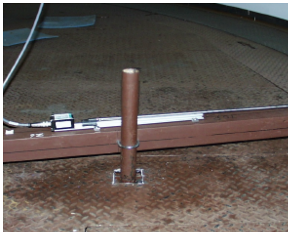
Figure 3.4 TLDT Mounted on Instrumentation Frame and Attachment to PCCV Liner
