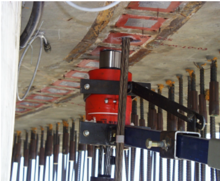
Figure 2.58 Tensioning Hardware Assembly and Load Cell
