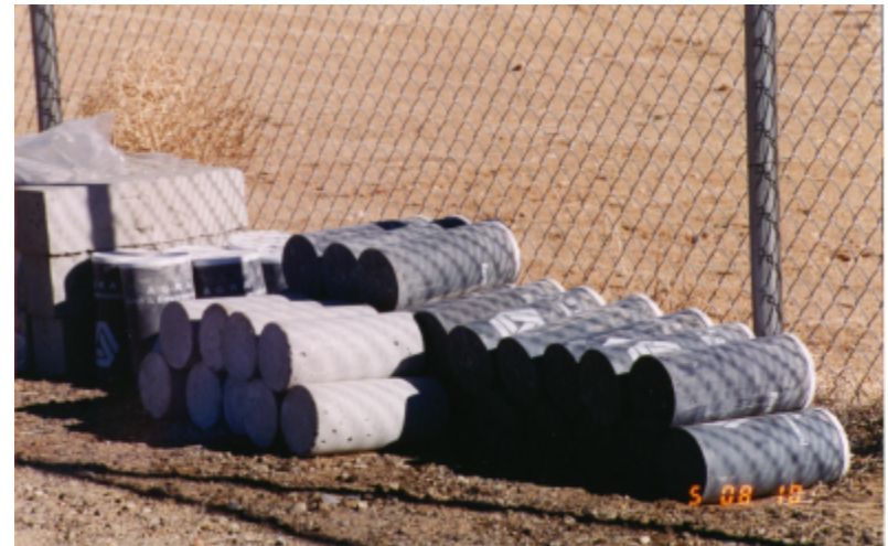
Figure 2.19 Concrete Test Cylinders and Beams
