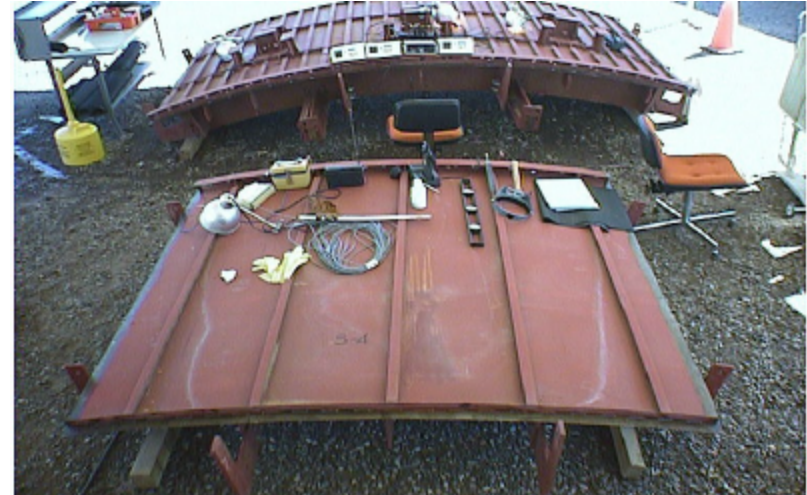
Figure 2.37 Liner Panel Instrumentation
