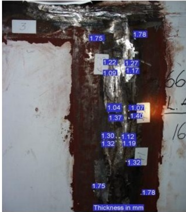
Figure 21. Liner thicknesses (in millimeters) measured ultrasonically in the vicinity of tear #4 (4-1, 4-2, and 4-3).
