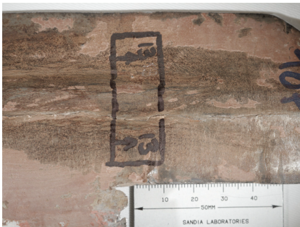
Figure 63. Details of inside (top) and outside (bottom) liner features in region #18-1 metallographic cross-section (arrows begin at plane of section and indicate view direction).
