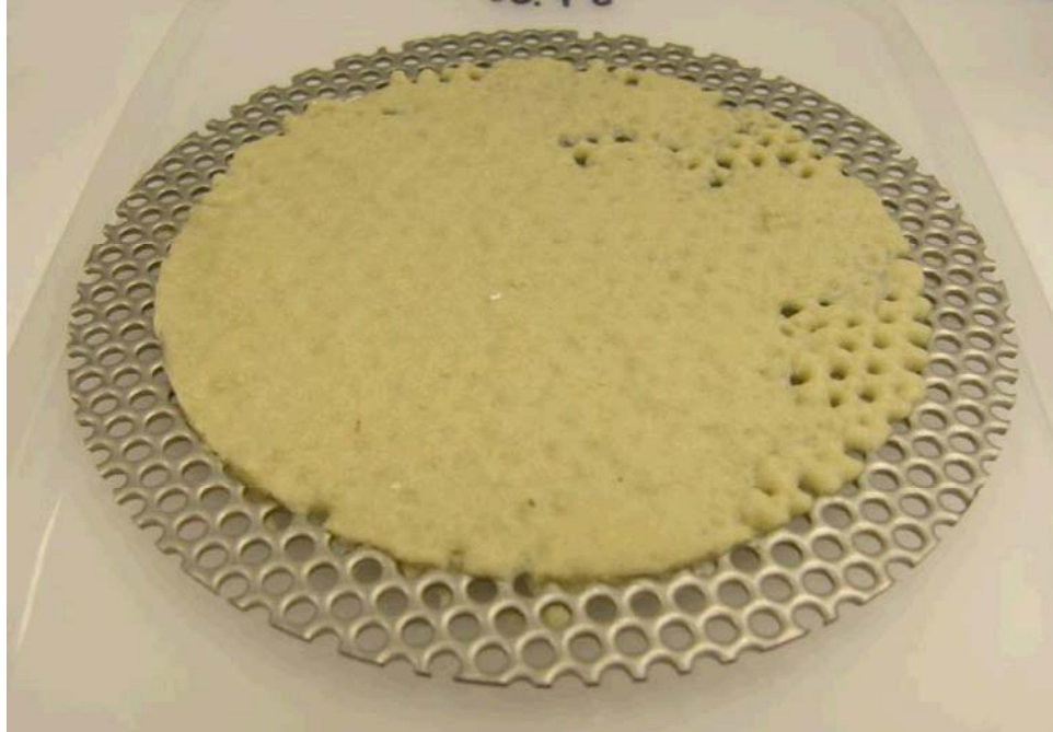
Figure 7.22. Incomplete Debris Bed from COBT2, Test 060510_CO_1469_BP1. Target CalSil mass loading = 1812 g/m 2 , retrieved CalSil mass loading = 237 g/m 2 , 13% of target mass retained on screen, debris bed formed in benchtop test loop.
