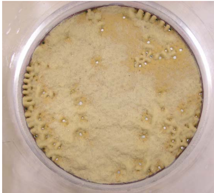
Figure 7.26. Incomplete Debris Bed from Test Condition CO1, Tests 060510_CO_8108_LP1 Through LP3. Debris bed pictured within TTS, target CalSil mass loading = 4350 \text{ g/m}^2 , retrieved CalSil mass loading = 434 \text{ g/m}^2 , 10% of target mass retained on screen, debris bed formed in large-scale test loop.
