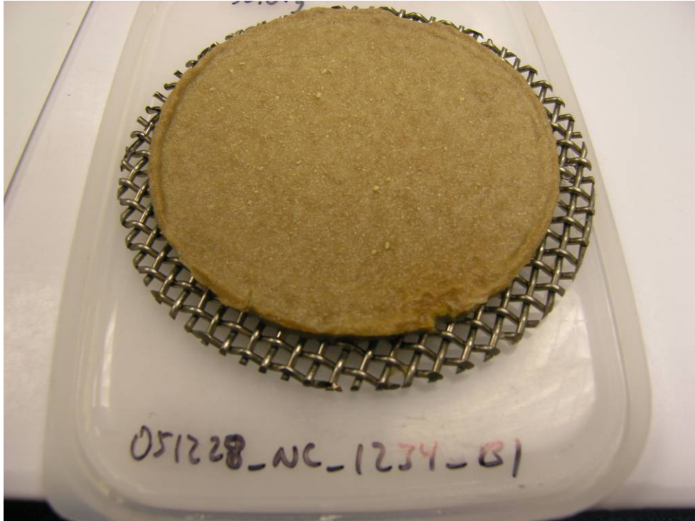
Figure 6.15. Test 051228_NC_1234_B1 NUKON/CalSil Debris Bed for Case 4A. Possible flow channel at 5:00 orientation.
