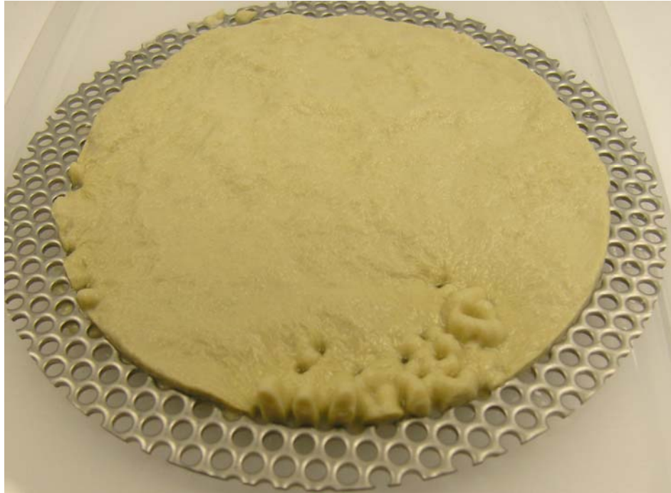
Figure 7.25. Incomplete Debris Bed from COBT7, Test 060511_CO_3527_BP2. Target CalSil mass loading = 4350 \text{ g/m}^2 , retrieved CalSil mass loading = 724 \text{ g/m}^2 , 17% of target mass retained on screen, debris bed formed in the benchtop test loop.
