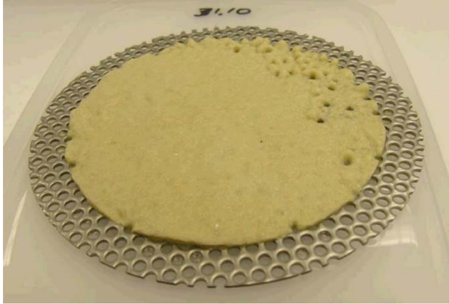
Figure 7.24. Incomplete Debris Bed from COBT6, Test 060510_CO_2351_BP3. Target CalSil mass loading = 2900 g/m 2 , retrieved CalSil mass loading = 390 g/m 2 , 13% of target mass retained on screen, debris bed formed in the benchtop test loop.
