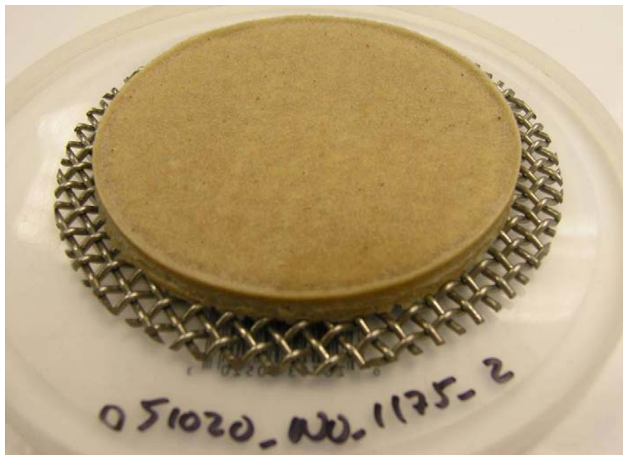
Figure 3.28. NUKON Debris Bed for R4D2 Subjected to 0.29 \text{ m/s} Screen Approach Velocity (target debris loading of 1449.5 \text{ g/m}^2 ; screen pattern perceptible on surface)
