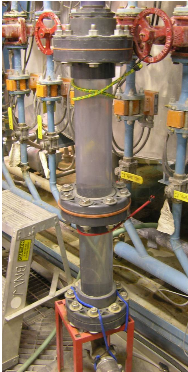
Figure 2.3. Photo of the Benchtop Loop Test Section. The test screen is sandwiched in the center set of pipe flanges.
