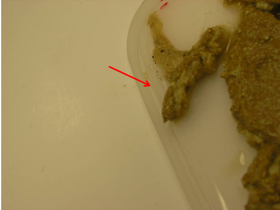
Figure 6.20. Test 051214_NC_1234_B2 NUKON/CalSil Debris Bed for Case 1B. Observation of CalSil Layer. Debris Bed Piece Tipped on Side. Brown “Specks” Are Rust From Loop Captured at Screen Surface.
