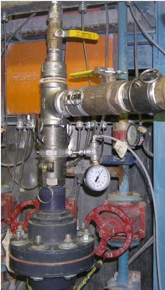
Figure 2.4. Upstream Portion of Benchtop Test Section Showing Pressure Tap Location
