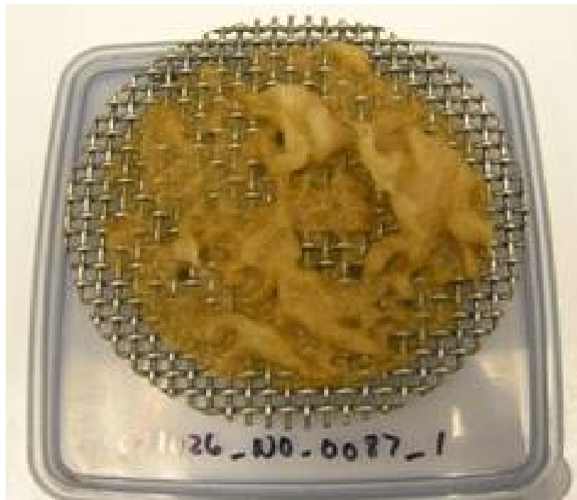
Figure 3.11. NUKON Debris Bed for 107.3 \text{ g/m}^2 Target Debris Loading (R4 ~ 20, no blender preparation)
