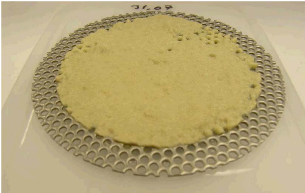
Figure 7.23. Incomplete Debris Bed from COBT5, Test 060510_CO_1763_BP2. Target CalSil mass loading = 2175 g/m 2 , retrieved CalSil mass loading = 292 g/m 2 , 13% of target mass retained on screen, debris bed formed in the benchtop test loop.
