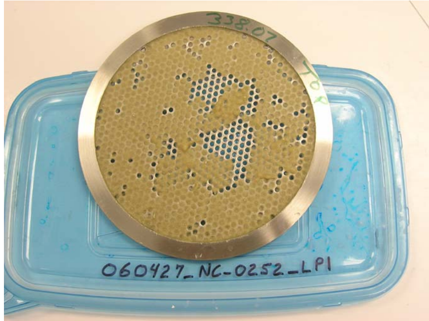
Figure 7.33. Incomplete Debris Bed Retrieved from Test NC1 with a Retrieved Mass Loading of 56.3 \text{ g/m}^2 . The target mass loading was 108 \text{ g/m}^2 NUKON, 27 \text{ g/m}^2 CalSil, and 135 \text{ g/m}^2 total.
