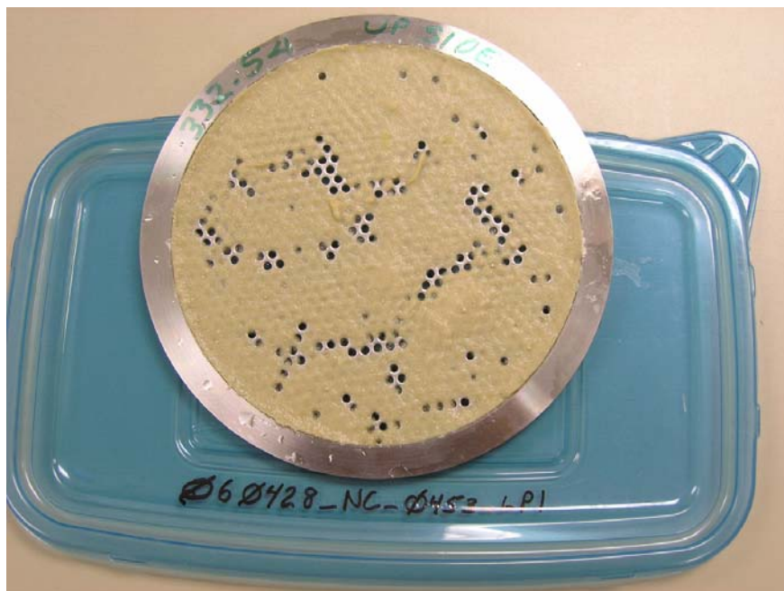
Figure 7.34. Incomplete Debris Bed Retrieved from Test NC2 with a Retrieved Mass Loading of 94.4 \text{ g/m}^2 . Target mass loading was 108 \text{ g/m}^2 NUKON, 135 \text{ g/m}^2 CalSil, and 243 \text{ g/m}^2 total.
