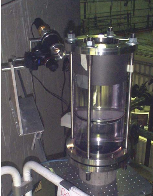
Figure 2.11. Photos of Optical Triangulation System Installed on the Large-Scale Test Loop
