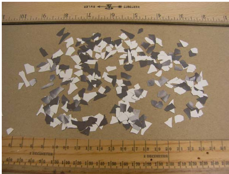
Figure 4.9. ¼-in. Square Coating ZE Coating Debris with Particle Dimensions of 0.157 to 0.265 in.
