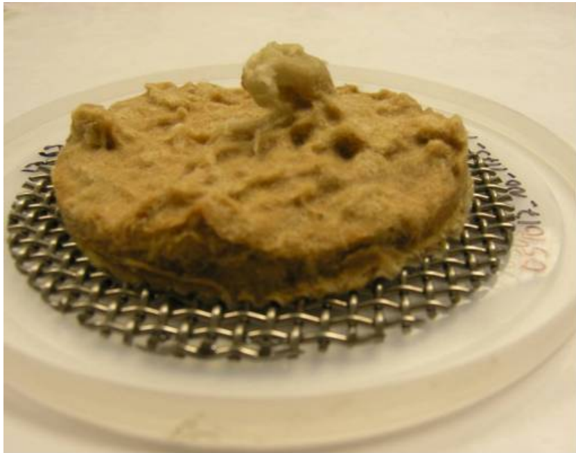
Figure 3.9. NUKON Debris Bed for 1449.5 g/m 2 Target Debris Loading (R4 ~ 17 as-received material/no blender preparation)
