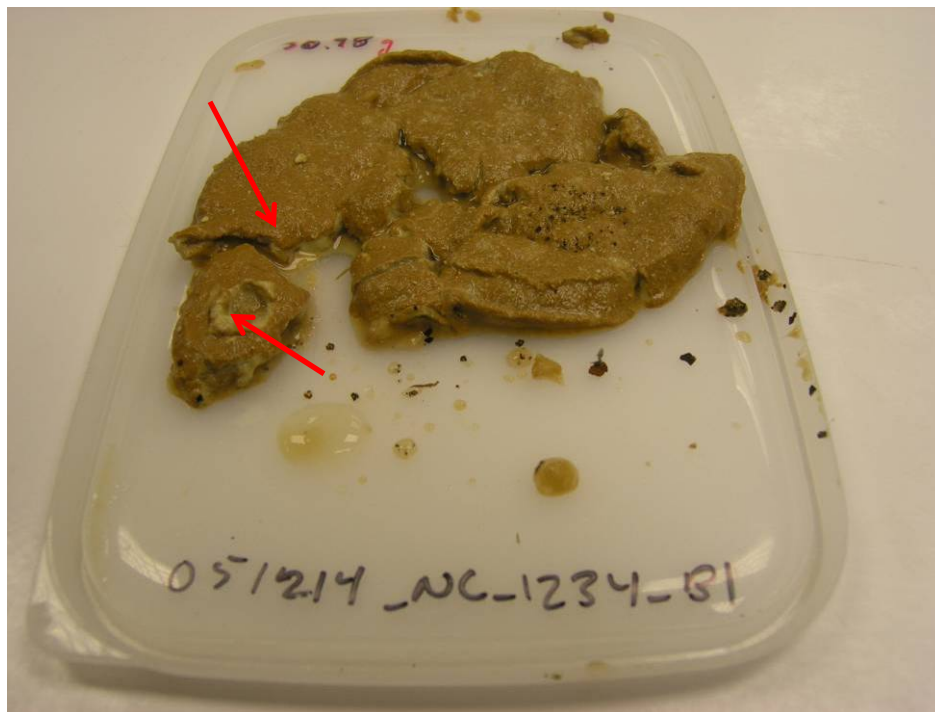
Figure 6.18. Test 051214_NC_1234_B1 NUKON/CalSil Debris Bed for Case 1A. Observation of CalSil Layer after attempt made to remove retrieved debris bed from the test screen. Brown “chunks” are rust from loop captured at screen surface.
