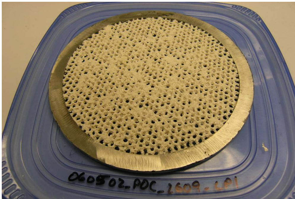
Figure 7.54. ALK2 Debris Bed After Retrieval from Test Section, Top View
