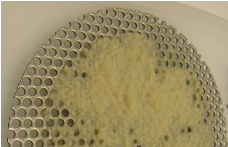
Figure 7.21. Incomplete Debris Bed from COBT1, Test 060406_CO_1176_BP1. NOTE: Debris bed was disturbed during retrieval. The lower half of the photo was not representative of the screen coverage achieved in the test loop and therefore was omitted from the figure. Target CalSil mass loading = 1450 g/m 2 , retrieved CalSil mass loading = 79 g/m 2 (reduced due to disruption of debris bed during retrieval), 5% of target mass retained on screen, debris bed formed in the benchtop test loop.
