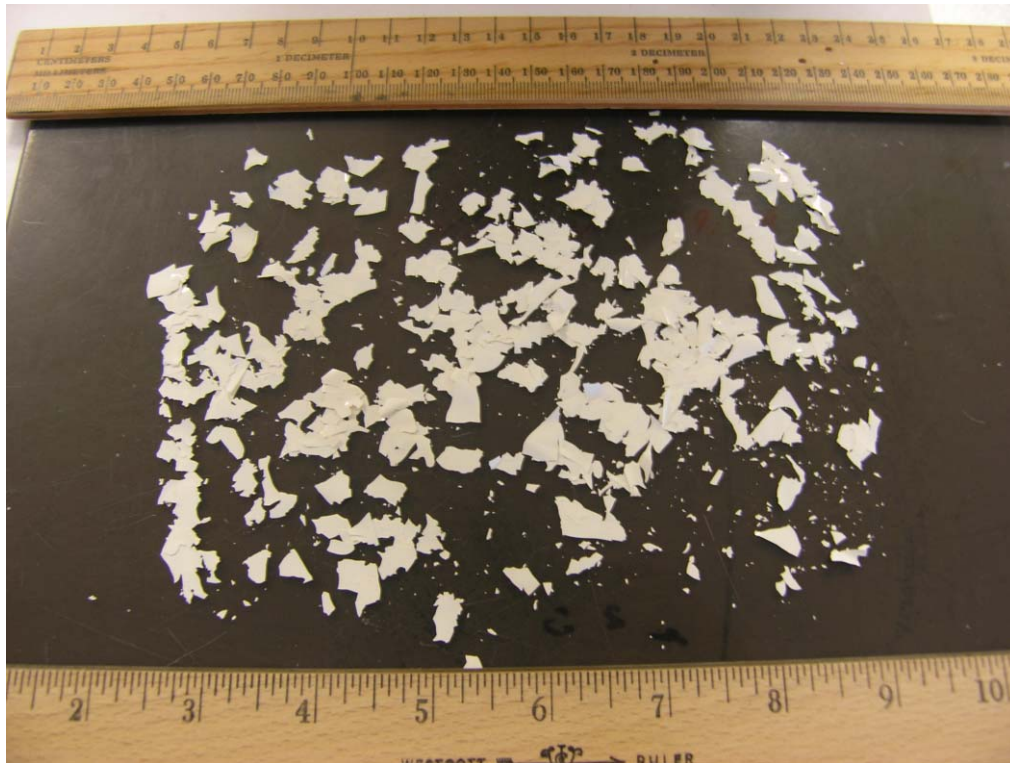
Figure 4.5. “1/4 in. Square Coating” (paint chips) for ALK Prepared Coating Debris in the Range 0.157 to 0.265 in.
