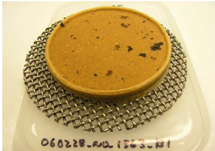
Figure 6.8. 060228_NO_1363_B1, 5-Mesh. Flakes are rust from benchtop loop components.
