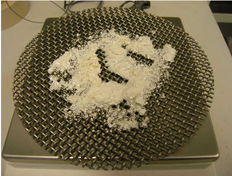
Figure 4.2. ALK Debris Poured onto 5-Mesh Screen for R4 Evaluation, R4 ~ 2.2
