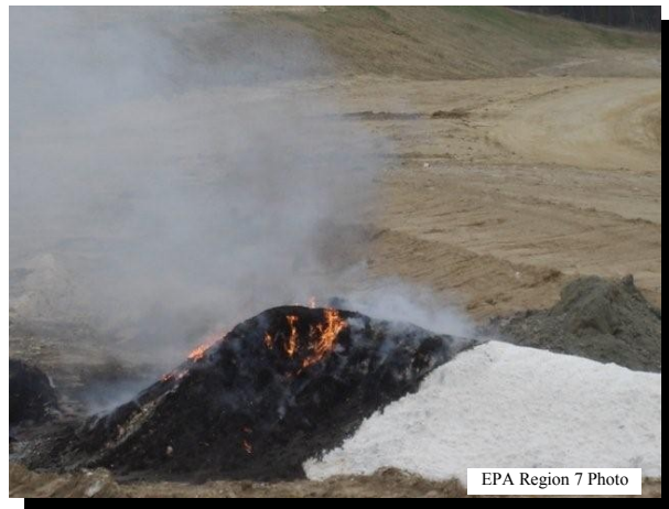
BIODIESEL FILTER MEDIA SPONTANEOUSLY COMBUSTING
