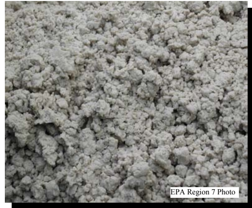
CLOSEUP OF DIATOMACEOUS EARTH WASTE
