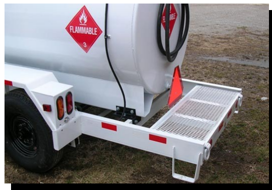
DIESEL FUEL TRANSFER TANK
