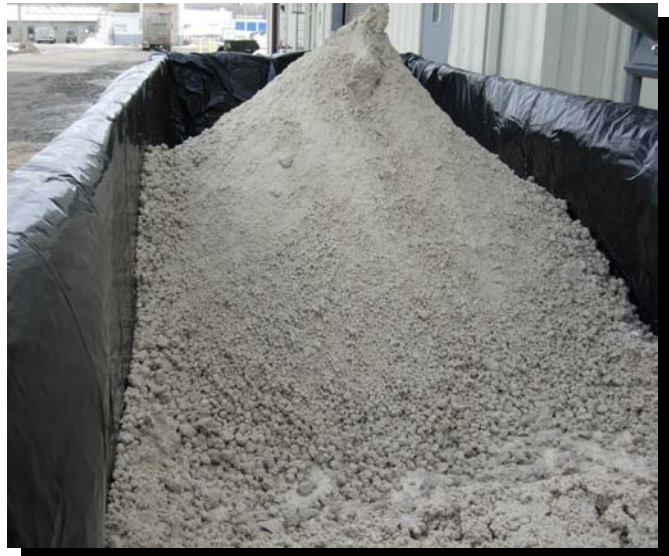
SPENT FILTER MEDIA FROM A BIODIESEL PLANT
