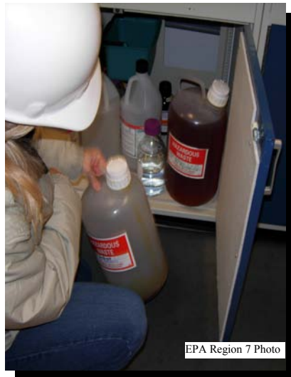
LABORATORY HAZARDOUS WASTE SATELLITE ACCUMULATION AREA
