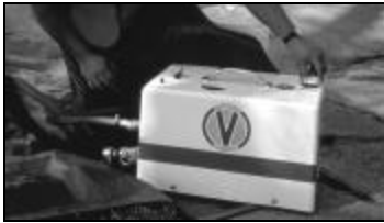
Figure 7-3. Small mixing equipment, such as the unit shown here, is used for foam treatment of lateral lines.
