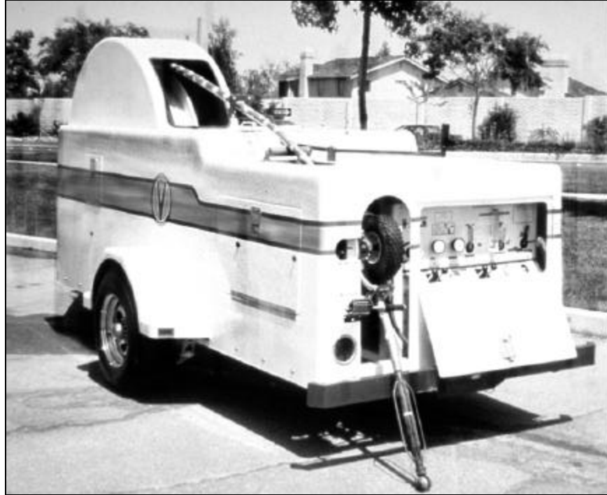
Figure 7-2. There are several types of equipment available for injecting foam root control pesticides into sewer systems.
