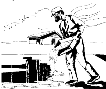
Figure 6-21. Build a dam of soil, cat litter, or other absorbent around the spilled material to keep it from spreading.
