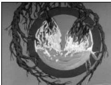
Figure 7-1. Although roots may be killed by pesticide treatment, it may take months or years for them to decay and leave sewer pipes.
