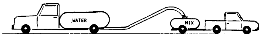
Figure 7-6. A sewer jetter provides a convenient source of water for filling application tanks and eliminates back-siphoning possibilities.
