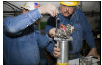
Technicians prepare a dynamic plutonium experiment, named Thermos, at the U1a facility 1,000 feet underground at the NTS. The Thermos experiments are designed to study damage to plutonium under dynamic stress conditions.
