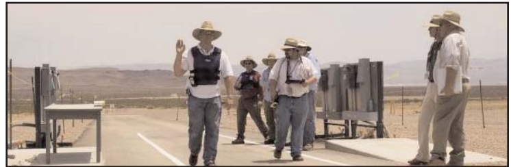
A PRD operator (simulating a law enforcement person) walks by a radiological source (on table). He has raised his hand indicating that the PRD has alarmed. The data is electronically collected by the 'tablet recorder' to the right of the operator. The test was called Pedestrian Surveying.
