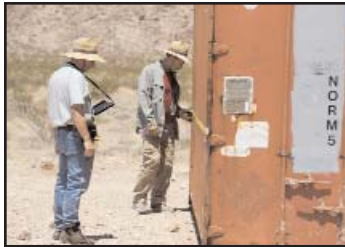
A PRD operator conducts an inspection of a cargo container holding a radiological source. The objective of this test called, 'Screening/Localization,' is to identify the exact location of the radiological source in the container. The data is electronically collected by the 'tablet recorder' to the left of the operator.
