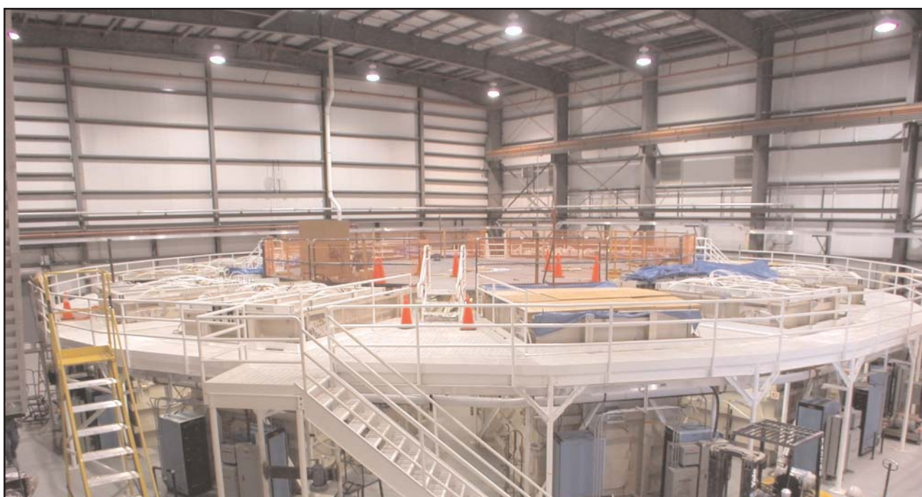
The Atlas machine at the Nevada Test Site is 80 feet in diameter and is comprised of a pulse power system which includes 12 Maintenance Units.
