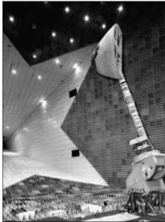
Development of spacecraft such as Apollo and the Shuttle required unusual and “unworldly” laboratories such as this anechoic chamber at JSC. The chamber replicates space by absorbing radio and radiation emissions.
