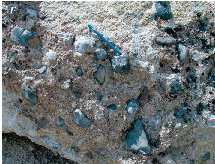
Figure 2 (continued). E , face of the Coal Creek No. 1 mine. Boulders in the lower left foreground are uranium-bearing conglomerates. F , uranium-enriched pebble-cobble conglomerate in the Coal Creek No. 1 mine. G , lower mine dump of Deer Strike claims. Composite mine-waste sample 11JH00 contained 140 ppm As, 540 ppm U, and 0.05 percent S.
