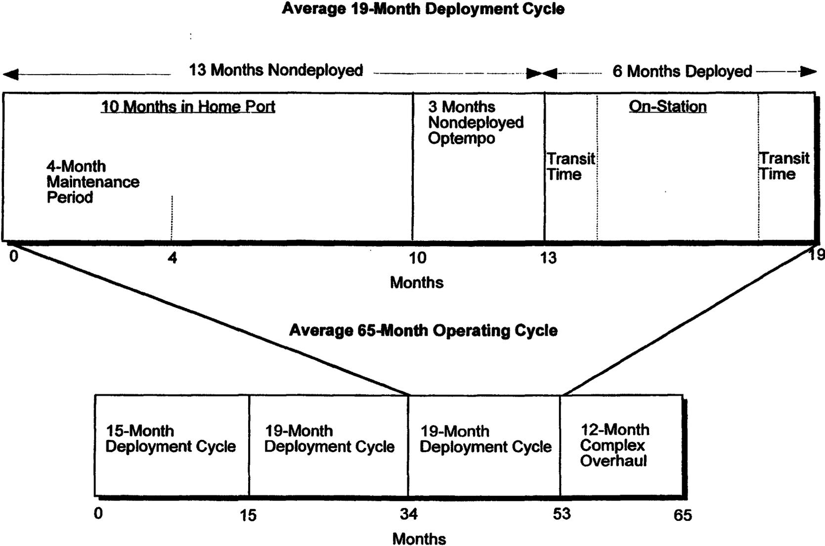
complete operating cycle for a conventionally powered carrier lasts about five and a half years.<sup>3</sup>
