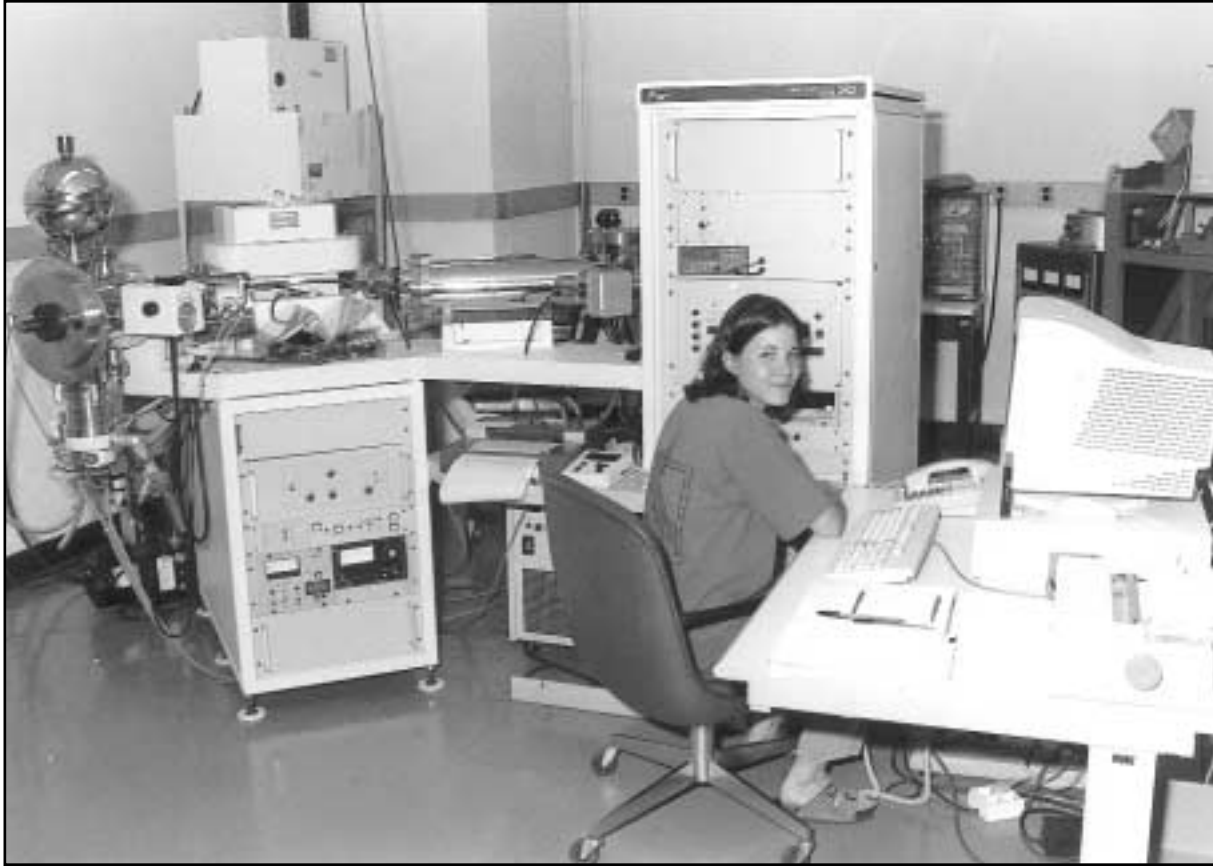
Automated, nine-collector Finnigan-MAT 262 mass spectrometer equipped with ion-counting capabilities. This spectrometer is used by the U.S. Geological Survey in Reston, Va., for automated analysis of lead, strontium, neodymium, uranium, thorium, rubidium, samarium, and boron. Isotopes of these elements are used to understand ore-forming processes and to date rocks.
