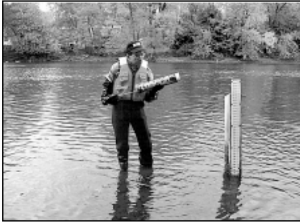
USGS scientist checking the Two Bridge gaging station and water-quality monitor on the Passaic River.
