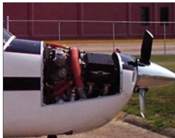
General Aviation Propulsion (GAP) piston engine aircraft installation.
