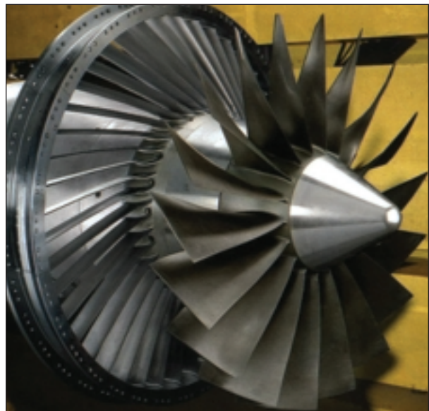
Swept and leaned strators—technology for noise reduction.
