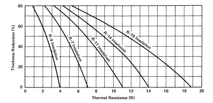
When insulation is installed over the framing members the thermal performance of the insulation is reduced due to compression at the framing members. The Resistance value of the insulation between the framing members is reduced by 12.5 percent for framing members 16" O.C., 8.5 percent for framing members 24" O.C., and 4 percent for framing members 48" O.C.
