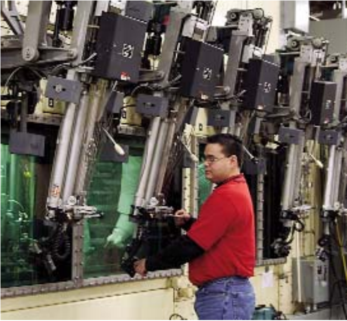
Space and Security Power Systems Facility (SSPSF), at Idaho National Laboratory, where radioisotope power systems are assembled
