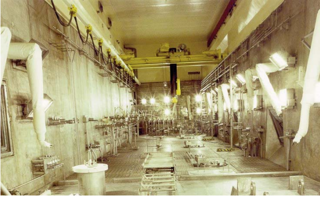
Fluorinel Dissolution Process cell at the Fuel Storage Area, Idaho National Laboratory
