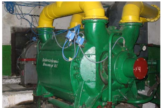
Figure 4. Vacuum pump for methane extraction used at the Bazhanov mine.
