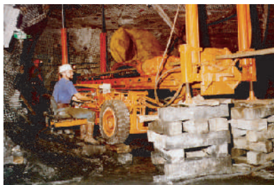
In-Mine Horizontal Drilling for CMM Capture. Photo courtesy of REI.
