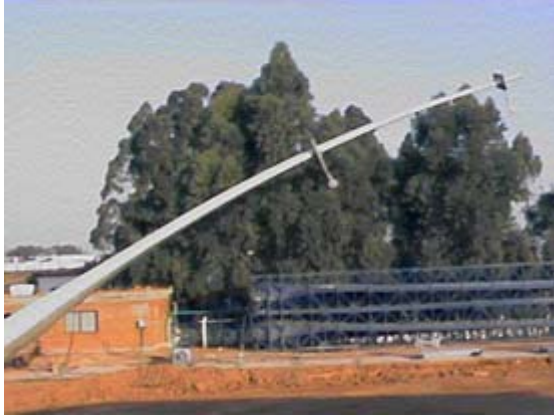
Figure 27. Static Blade Tests
