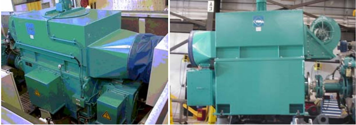
Figure 19. POC Water-Cooled Loher 1.5-MW Generator
