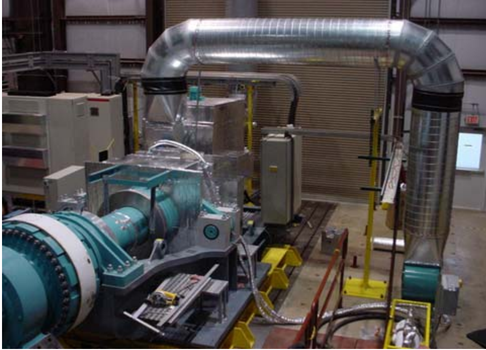
Figure 21. POC Drive Train on the NWTC Dynamometer Test Stand
