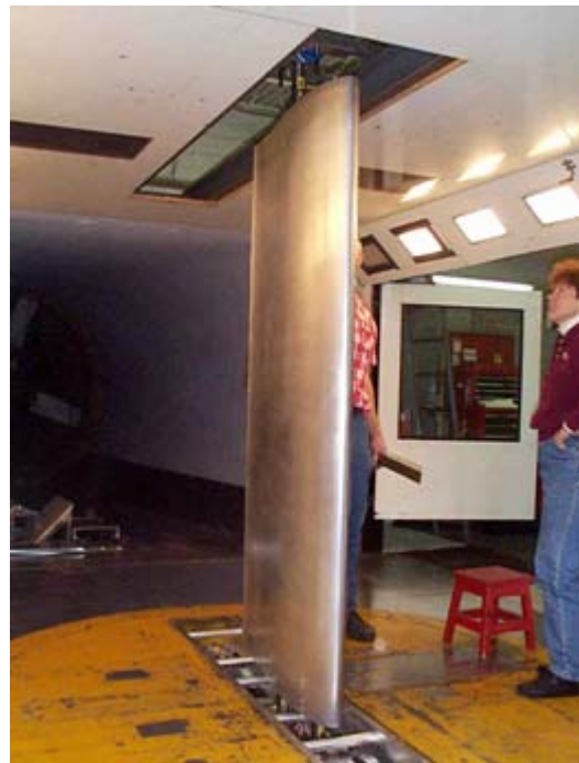
Figure 25. 18% Airfoil Model in the WSU Wind Tunnel Test
