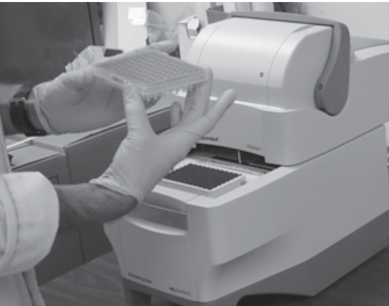
Figure 5. Experiments are under way at the park to determine the concentration of enterococci, a fecal coliform bacteria, using quantitative PCR. This technique can potentially measure fecal indicator bacteria in less than two hours compared to the 24-hour test now in use.
