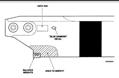
Figure 1. Tail rotor blade inspection.
