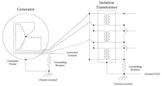
Note that the grounding resistor must be mounted on the same frame with the generator.
