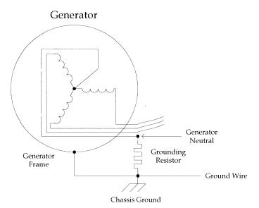
Note that grounding resistor must be mounted on the same frame with the generator.
