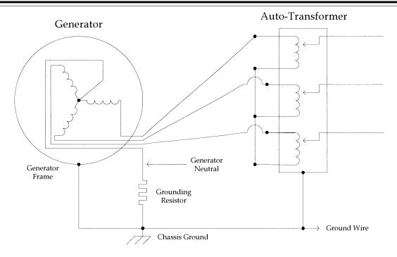
Note that the grounding resistor must be mounted on the same frame with the generator.
