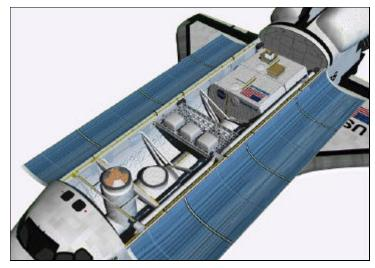
Spacehab Double Cargo Module in Shuttle payload bay
