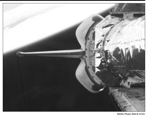
The Chandra X-Ray Observatory, the world's most powerful X-Ray telescope is shown in Columbia's payload bay before its deployment by the STS-93 crew.
