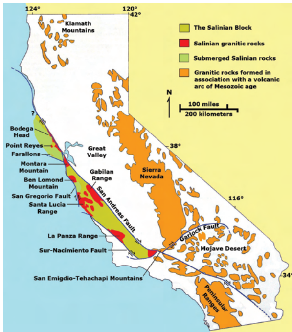
Figure 8-20. Map showing granitic bedrock provinces of California highlighting the extent of the Salinian Block. Exposures of granitic bedrock in the Salinian Block are shown in red. The Salinian Block extends offshore to the shelf margin to some undetermined extent north and west of the San Francisco Bay Area. The block is bounded on the east by the San Andreas Fault and on the west in the southern part by the Sur-Nacimiento and San Gregorio Fault systems. The western side of the northern Salinian Block is probably bounded by faults in the offshore region along the continental shelf margin.
