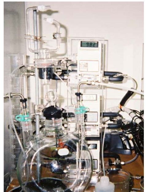
In the foreground is a glass vessel used to supply interferent vapors—for example, paint fumes for testing.
