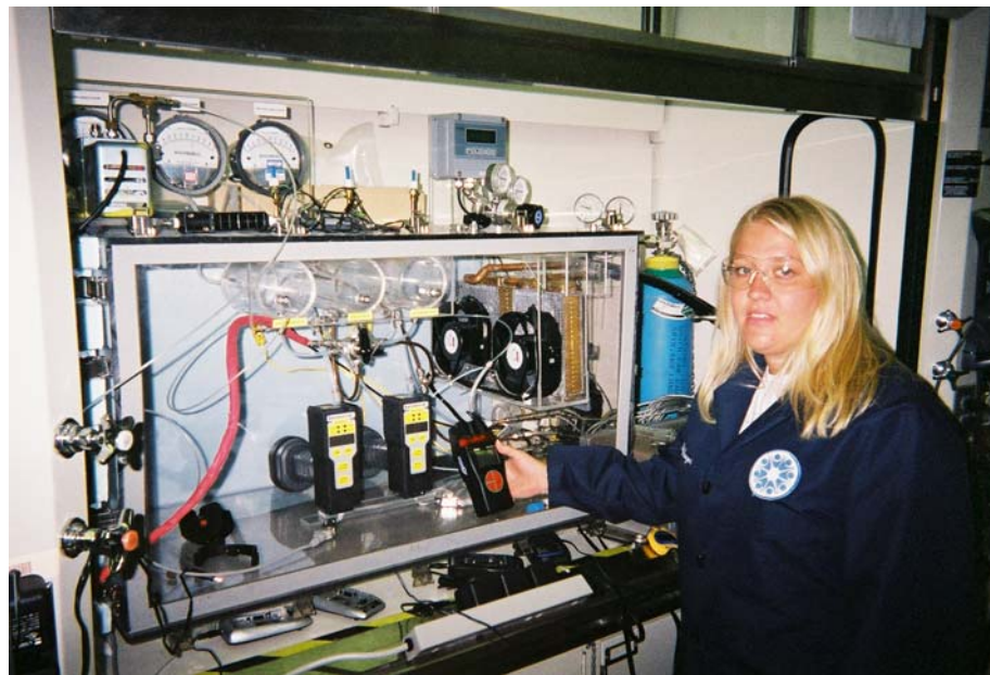
Two HAZMATCAD Plus instruments submitted for testing by Microsensor Systems, Inc. (at left), are being tested by Battelle's Robyn Kroeger, who is using an electrochemical device to perform an independent check of the concentration of a TIC, in this case, chlorine.
