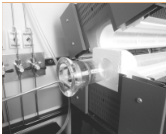
NCPV research at NREL led to this annealing technique for heat treating CdTe solar cells to improve performance and manufacturing.
