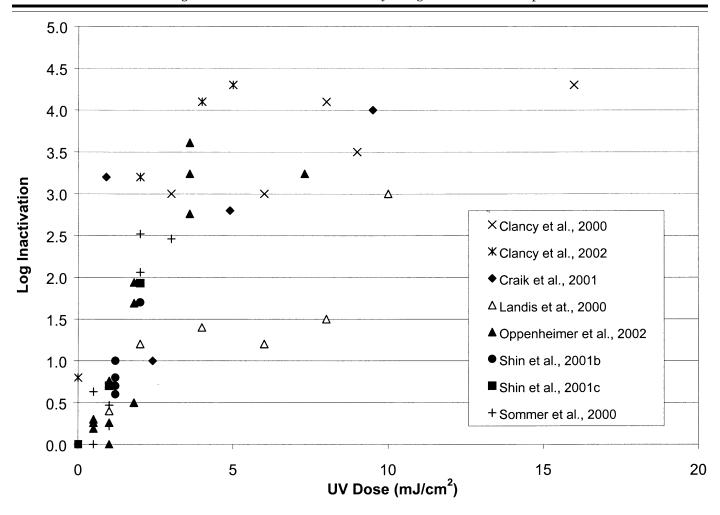
Figure III-5.-- Inactivation of Cryptosporidium by UV Light
