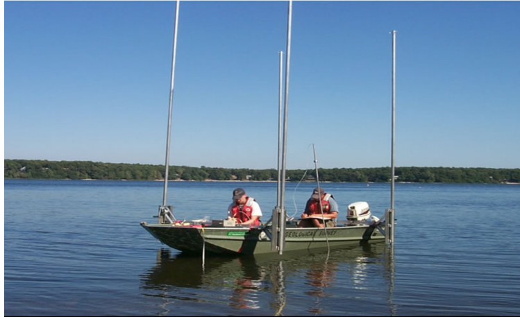
As part of the toxic substances hydrology program, USGS scientists collect ground water samples from the pond bottom at Johns Pond, Cape Cod, Massachusetts, with a drive-point sampling well to confirm data obtained with diffusion samplers.
