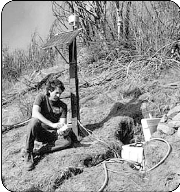
Testing a solar-powered radio telemetry system for remote transmission of real-time landslide data. Photograph by Mark Reid, USGS.
