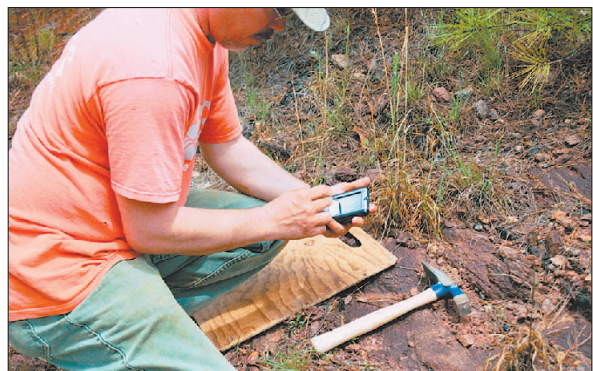
The USGS, working with Dr. Randy Kath of the State University of West Georgia, has developed a system for digital collection of structural data using a handheld computer and a global positioning system receiver. The photo above shows structural data being entered at a quartzite-schist outcrop. Photo by Ethan W. Williams.
