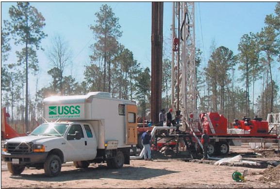
C. A logging truck collecting geophysical logs, and a hydraulic rotary drill rig at a well in Chatham County. As part of the Coastal Sound Science Initiative, geophysical, geologic, and water-quality data are collected from test wells drilled by the USGS and from wells drilled by private citizens. Photo by Michael F. Peck, USGS.
