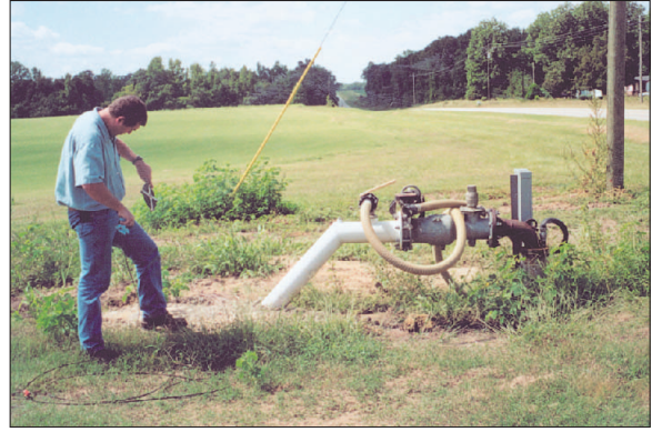
B. A USGS employee using a graduated steel tape to measure the water level in an irrigation well in Burke County. Periodic water-level measurements were made in 257 wells throughout the State during 2001. These measurements are used to construct potentiometric-surface maps for selected aquifers. Photo by Michael D. Hamrick, USGS.
