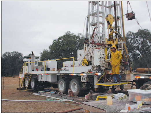
A 1,863-foot-deep exploratory boring was completed at a site in northern McIntosh County during 2001. Geologic, hydrologic, water-quality, and geophysical data are being evaluated to assess the viability of the Lower Floridan aquifer as a source of water and to support ground-water modeling investigations in coastal Georgia. In addition to the McIntosh County well, two additional wells were completed in Bryan and Effingham Counties during 2001. Photo by John S. Clarke, USGS.
