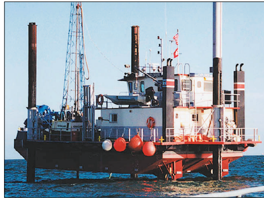
The U.S. Army Corps of Engineers jack-up barge was used as a platform for drilling offshore test borings. Core, hydrologic, water-quality, and geophysical data were collected at five sites during 1999–2001. Data are being used to investigate the position of the freshwater-saltwater interface and to better define hydraulic head and hydraulic properties offshore of Tybee Island, Georgia, and Hilton Head Island, South Carolina. Photo by Michael F. Peck, USGS.
