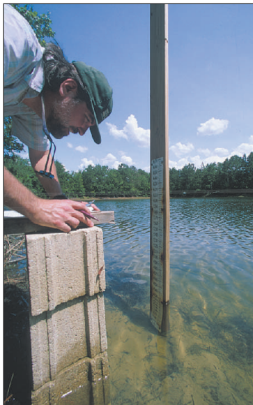
A USGS hydrologic technician takes a stage reading at a seepage pond in Bulloch County during a pumping test during May 2001. The test is being conducted to assess the viability of seepage ponds as an irrigation water supply. Test sites at Bulloch and Glynn Counties were instrumented with test wells, weather stations, and stage recorders to develop a detailed hydrologic budget and determine pond-aquifer relations. Photo by Alan M. Cressler, USGS.
