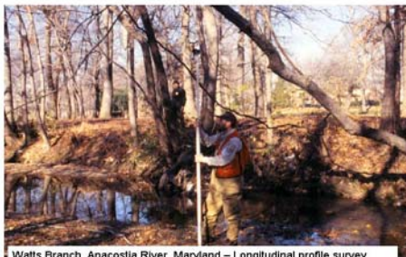
Watts Branch, Anacostia River, Maryland – Longitudinal profile survey used to characterize stream bed (i.e., pools, riffles, runs, and glides)
